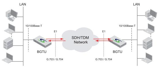
Typical application: Interface Converter fractional E1 + nx64 kbit/s ↔ G.703 / G.704 (E1)
